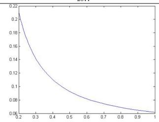
Figure 6: The Diagram of Occurrence - Severity for Lognormal Distribution
