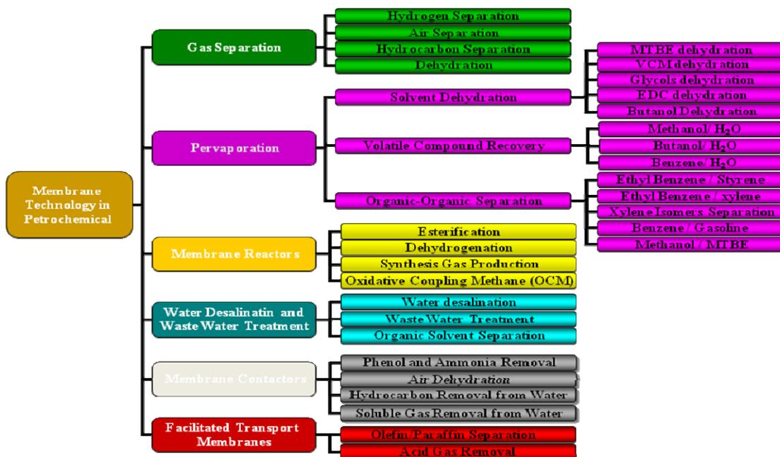
Fig 3: First level of Membrane technology process map in petrochemical industry
