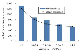
Figure 2 Nitrogen Foam Profile Production Effect for Different Crude Oil Viscosity
