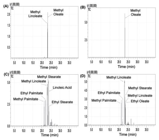
Figure 3 Chromatogram with Mass Spectrum Identification for Biodiesel Sample (A) Methylic Corn Waste Oil, (B) Methylic Canola Waste Oil, (C) Ethylic Corn Waste Oil, (D) Ethylic Canola Waste Oil
