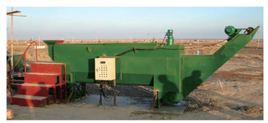
Figure 4 On Site Small-Size Horizontal Hot Water Separation Devices for Oil Sand
