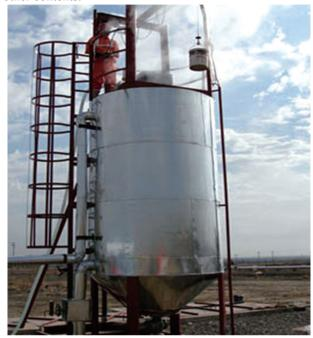
Figure 3 On Site Small-Size Vertical Hot Water Separation Devices for Oil Sand
