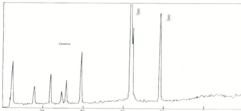
**Fig. 8: X-ray Diffraction Pattern for White Sand of Um Bogma**
