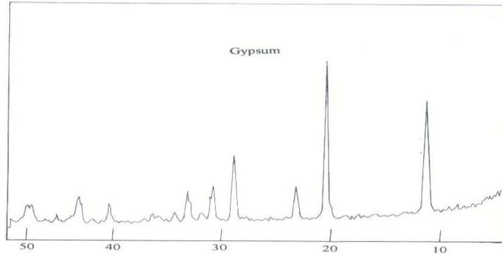
**Fig. 7: X-ray Diffraction Pattern for Gypsum of Ras Mallab**
