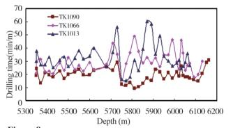
Figure 8 Drilling Time Comparison of TK1090 and Adjacent Well
