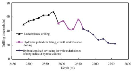
Figure 11 Comparison of Jinlong 3 Well Test Interval and Adjacent Interval
