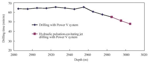
Figure 12 Comparison of Fengcheng 1 Well Test Interval and Adjacent Interval
