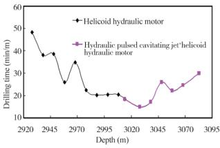
Depth (m) Figure 9 Drilling Time Comparison of Wu 34 and Adjacent Well
