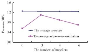
Figure 6 The Curve of Pressure Oscillation and Impeller Number
