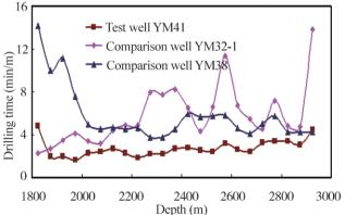
Figure 10 Drilling Time Comparison of Yingmai 41 and Adjacent Well
