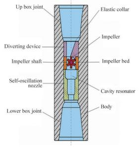
Figure1 Structure of Hydraulic Pulsed Cavitating Jet
