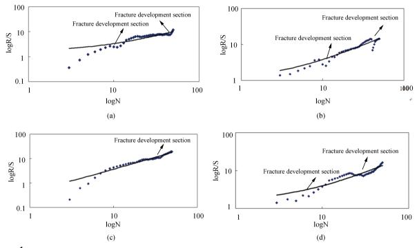
Figure 1 The Double Logarithmic Relationship Diagram Between R/S and n of the Amplitude Difference Data. (a) Su53-4, Depth Interval: 3,229.735 - 3,235.860 m, (b) Su53-8, Depth Interval: 3,168.25 - 3,174.375 m, (c) Su 53-78-46H, Depth Interval: 3,475.625 - 3,481.75 m, (d) Su 53-78-58H, Depth Interval: 3,395.825 - 3,401.95 m
