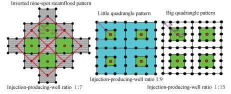
Figure 6 Schematic Diagram of Different Wells Network Solution
