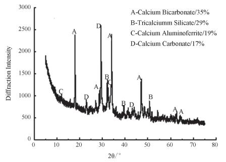
Figure 7 Component Diagram of the Puree Cement Stone After Corrosion
