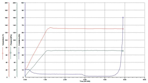
Figure 1 130 °C × 70 MPa Supercharging Thickening Curve Note. Shengwei glass G 593 g + silicon powder 207 g + water 275 g + SWJ-3 24 g + SWJZ-1 3.2 g + SDJR 40 g + SDW 2 g + SWH-1 2.8 g + salt 33 g + antifoaming agent 2 g.
